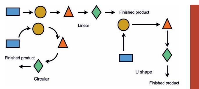
**Figure 2** – *Example of work cell layouts* (Source: adapted after Black & Hunter, 2003)
